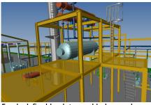
Freely definable plates and holes can be added to steel structures
